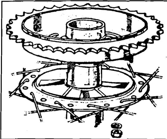
If the cush drive rubbers are worn, and the amount of free movement measured at the tyre exceeds 1/2" to 1", the rubbers should be replaced. The condition of the cush drive rubber in the rear wheel can be gauged by placing the machine on the rear stand, applying the rear brake and rotating the rear wheel.
