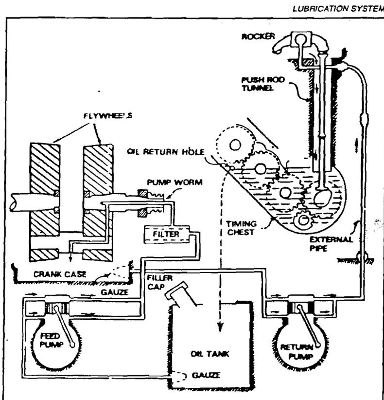
Both pumps are double acting, but two sides of feed pump are inter-connected, thereby giving an augmented and even supply to the big-end. Return pump is also inter-connected for effective scavenging from crank case.
