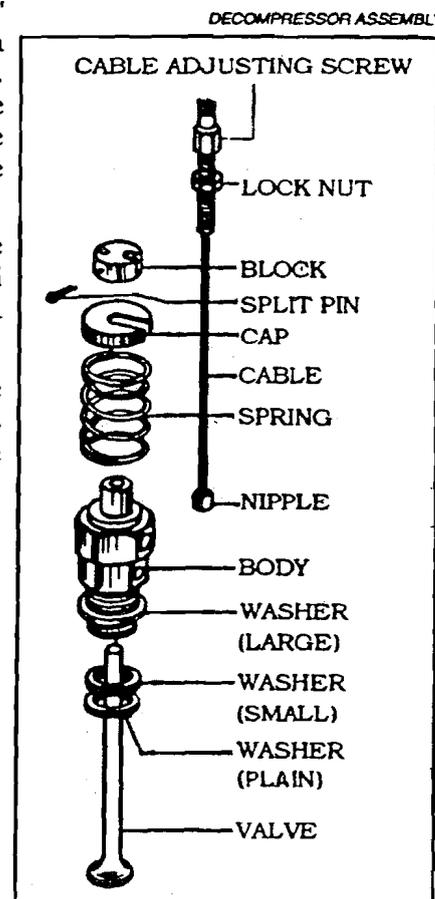
upwards and pull the cable nipple out of the body. It will now be possible to remove the cable and nipple through the spring, leaving the decompressor body and spring detached from the control cable.
