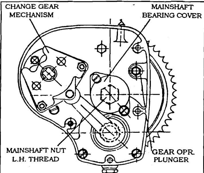
*The gear box is bolted on to the back of the crankcase and has fourspeeds, which are foot-controlled, and a patented neutral finder. All gears are in constant mesh, changes being effected by robust dog clutches.*
