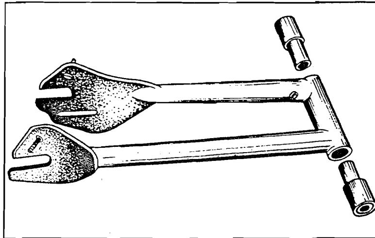
position of the spring box. The special tool for alignment of swing arm to be used. (PED 2044). No maintenance is necessary for the swinging arm pivot.
