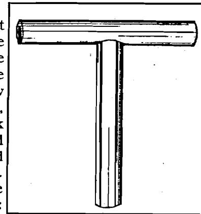
Now unscrew the main tube valve port using special tool PED 2026. The spring stud and spring can now be withdrawn from the lower end of the main tube.
