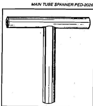
Now unscrew the main tube valve port using special tool PED 2026. The spring stud and spring can now be withdrawn from the lower end of the main tube.
