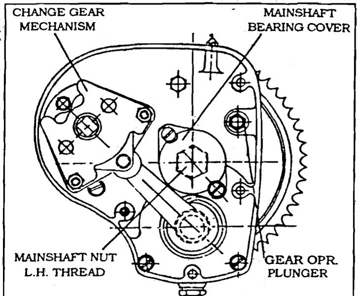
The gear box is bolted on to the back of the crankcase and has four speeds, which are foot-controlled, and a patented neutral finder. All gears are in constant mesh, changes being effected by robust dog clutches. The internal gear ratios are 2.77 : 1 (1st Gear), 1.84 : 1 (2nd gear) 1.36 : 1 (3rd gear) and 1 : 1 (Top gear)
