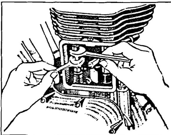
Proceed as follows for adjustments. Bring the piston to TDC at the end of compression stroke, so that both the valves are at the closed position. This may be ensured by seeing the valve timing marks, if the timing cover is open or through ammeter needle in its centre position, when ignition is switched on.
