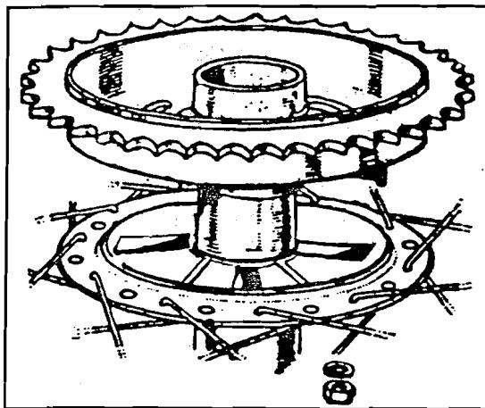
If the cushion drive rubbers are worn, and the amount of free movement measured at the tyre exceeds  $1/2"$  to  $1"$ , the rubbers should be replaced. The condition of the cushion drive rubber in the rear wheel can be gauged by placing the machine on the rear stand, applying the rear brake and rotating the rear wheel.
