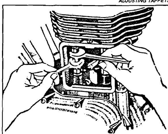
Proceed as follows for adjustments. Bring the piston to TDC at the end of compression stroke, so that both the valves are at the closed position. This may be ensured by seeing the valve timing marks, if the timing cover is open or through ammeter needle in its centre position, when ignition is switched on.
